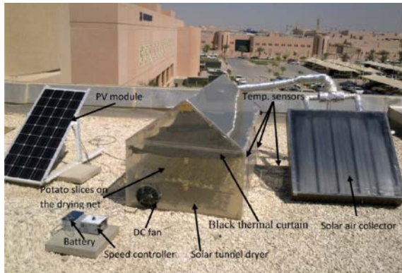
Fig. 7. Photograph of hybrid PV solar tunnel dryer for potato chips.
